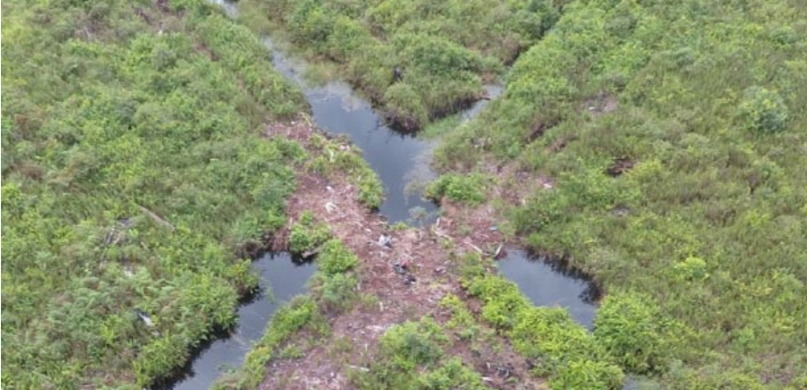
Figure 3-12b (below): A medium canal in conservation area in West Kalimantan blocked with compacted peat dam constructed by excavator.
