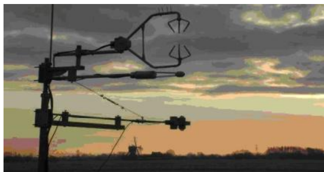
Figure 5. An eddy covariance system, equipped with sensors for irradiation, wind, temperature, CO_2 and water vapour (Photography E. Veenendaal).
