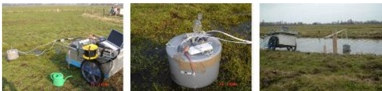
Figure 2. An example of a portable enclosure, connected to a gas analyser and a computer (a). The enclosure is equipped with a water lock to avoid pressure differences and a filter for water vapour to avoid cross-interferences (b). The system can be used to measure CO 2 , CH 4 and N 2 O on land or on water (a and c) (Photography A. Schrier-Uijl)
